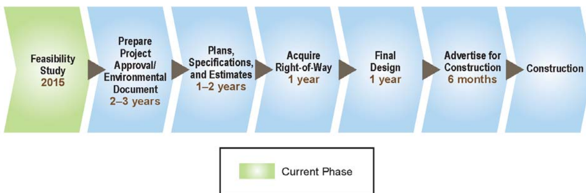
Figure 5. Typical Project Development Schedule
